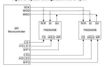
Figure 2. System Configuration with SPI port
