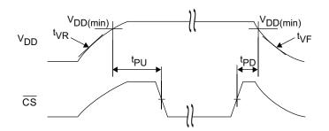
$<sup>\</sup>label{eq:Note} \textbf{12. Slope measured at any point on $V_{DD}$ waveform.}$
